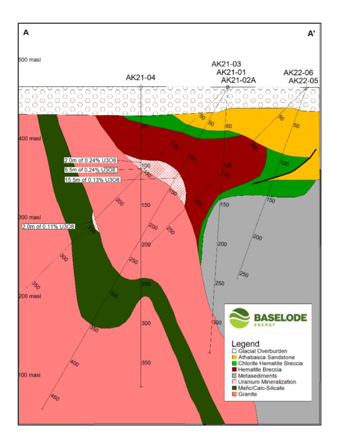
FIGURE 3 – Geology schematic cross-section of drill holes AK21-01 to AK22-06 (view looking north)
