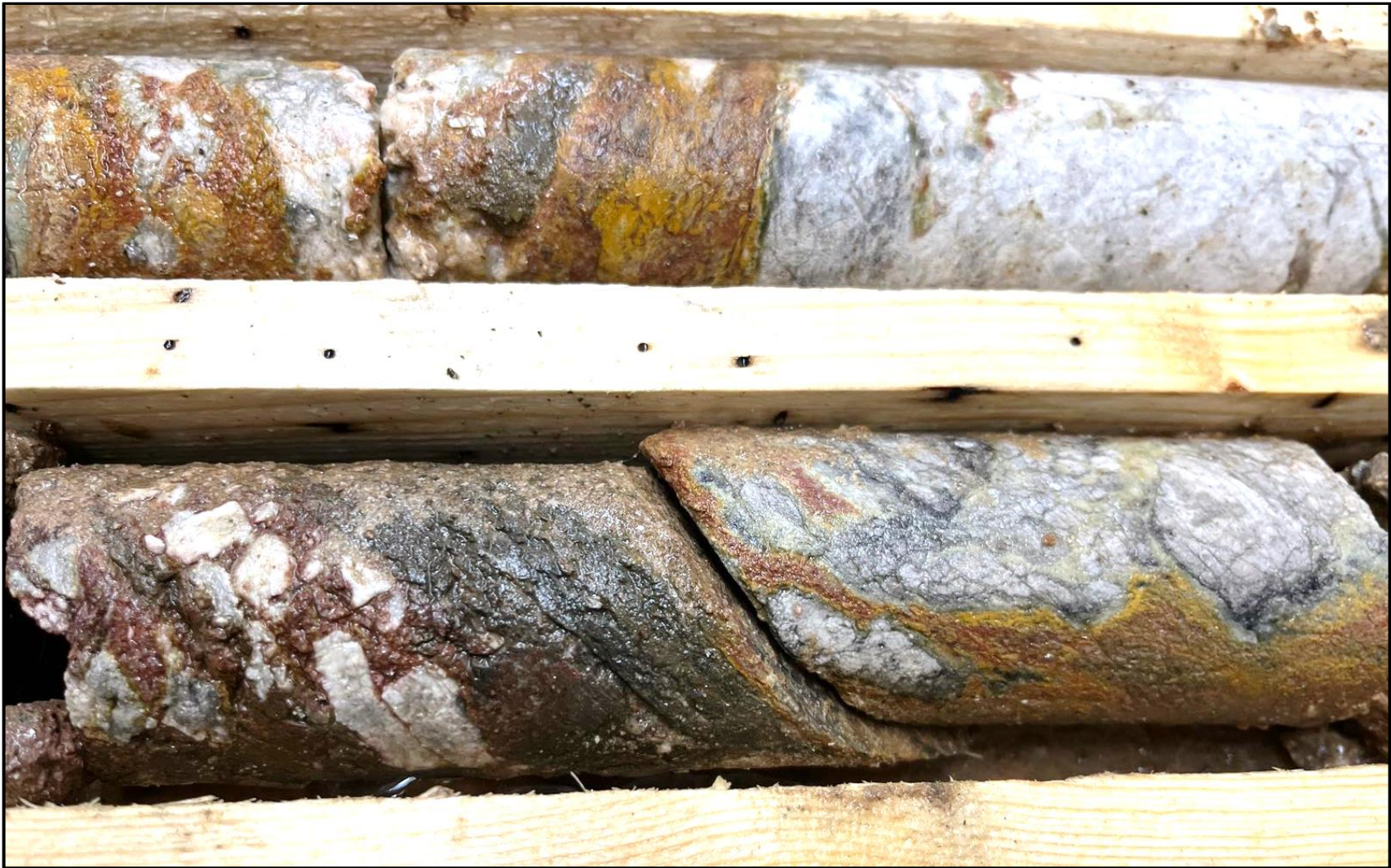
FIGURE 6 – CT24-011, 144.3 m depth, close-up of redox-style hydrothermal alteration
