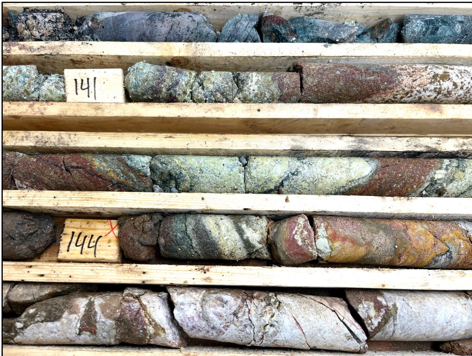
FIGURE 5 – CT24-011, 138.5 to 145.5 m, close-up of clay and redox-style hydrothermal alteration
