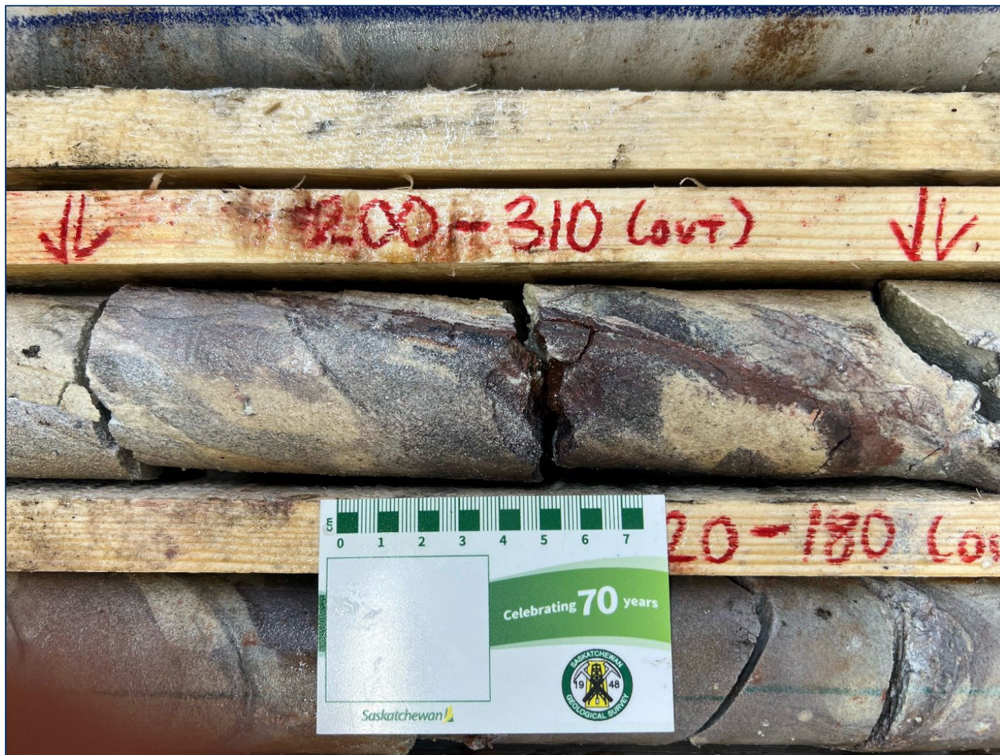
FIGURE 5 – Fracture-controlled, hydrothermal remobilized anomalous radioactivity, HK24-016
